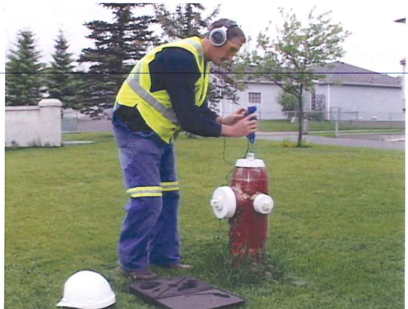
A distribution systems operator performs leak detection tests in Okotoks, Alberta
